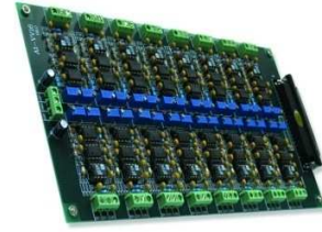
CONDITIONING TERMINAL BOARD
